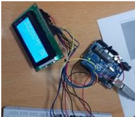
Figure 4: Arduino & LCD connections
