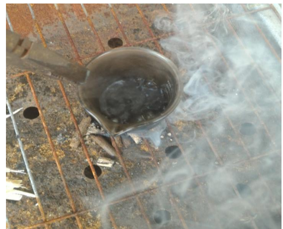
Figure 3: Water in beaker B which is heated by oil palm waste starts to boil
