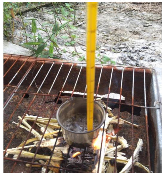
Figure 2: Water in beaker A which is heated by sugarcane bagasse starts to boil
